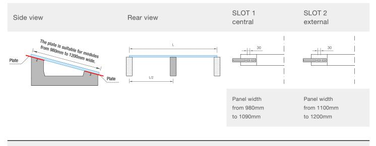
USE ONE OF THE TWO 30MM SLOTS TO FIX THE PLATE ON THE CENTRAL REINFORCEMENT BALLASTS, DEPENDING ON THE PANEL WIDTH
