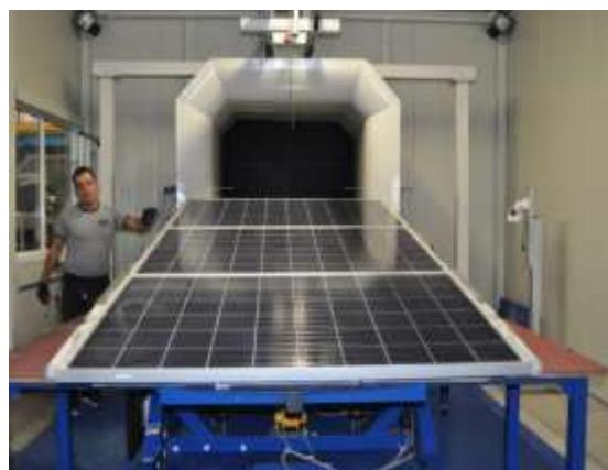
**ID 38: Model 11° "Sail" Configuration 2/3 with accessory plate to joint ballasts**
