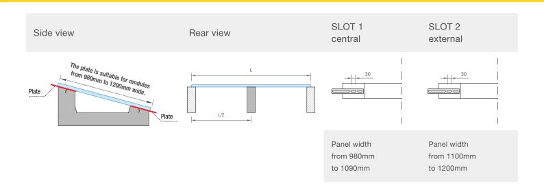
USE ONE OF THE TWO 30MM SLOTS TO FIX THE PLATE ON THE CENTRAL REINFORCEMENT BALLASTS, DEPENDING ON THE PANEL WIDTH
